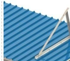
**Step2.** Install mounting rail on triangle legs by L-feet
